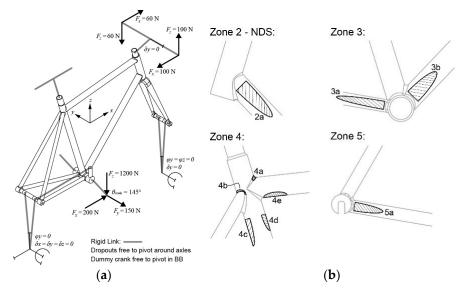
**Figure 2.** A recent example of modelling and simulation on steel bicycle frames: (**a**) FEA has been applied to bicycle frames with load cases based on field measurements [3]; (**b**) Areas of high stress for specific load cases can be identified and evaluated [3].
