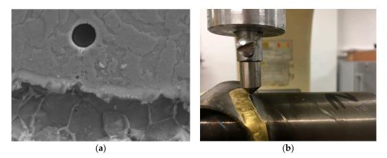
**Figure 3.** (a) Scanning electron microscopy (SEM) at the bimetallic bond between steel and brass (Cu60%, Zn38%). The strength of this interaction (i.e., the chemical compatibility) will determine the strength of the joint and the minimum fillet size; (b) Tests to determine the hardness in the heat-affected zone (HAZ).
