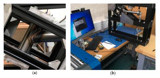
**Figure 4.** The authors have developed a prototype test rig that will allow for welded and brazed bicycle frame joints to be tested for their static and fatigue strengths: (**a**) the method of fixation using a set of customised expanding arbors; (**b**) loads can be applied using hung masses or stepper motor or pneumatic cylinder.
